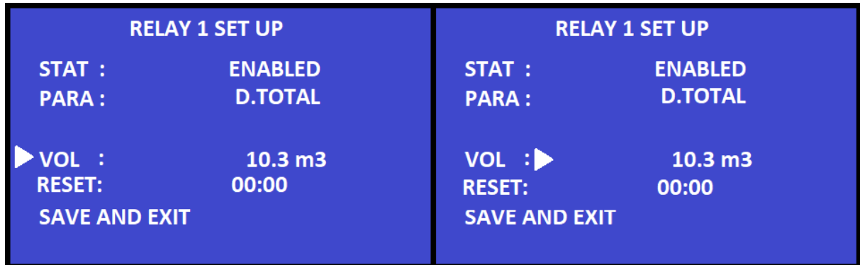
Figure 15-4 Daily Totaliser Relay Set Up
