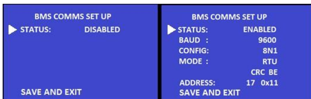
Figure 12-1 Modbus BMS Set Up
