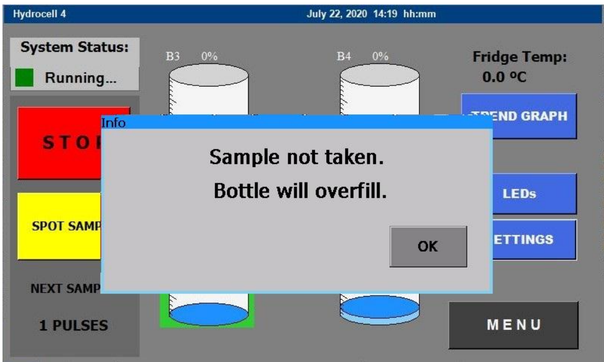
Figure 5.3.1 HC4 Bottle requires Emptying
