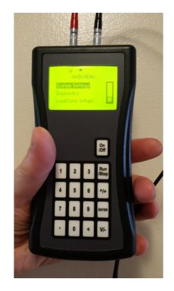
The POCKET-UFM is a light weight, truly pocket sized instrument. Its intuitive menu driven HMI makes it incredibly easy to use. Its size and the layout of its display and keypad means that it can be operated single handed. Yet all of this is achieved with no compromise in measurement performance. It even incorporates wall thickness and heat quantity measurement functionality.
